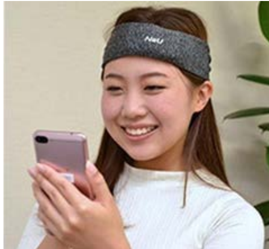
Figure 2 The participants wore a precharged XB-01 with a headband a little over the left eyebrow on the forehead. Copyright by NeU Inc.
